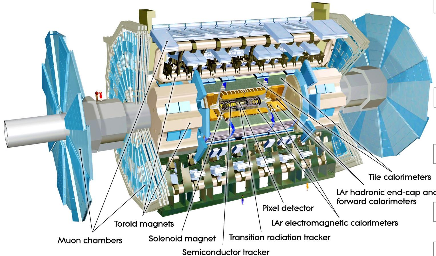
25 m diameter, 44 m long, 7000 tons weight
