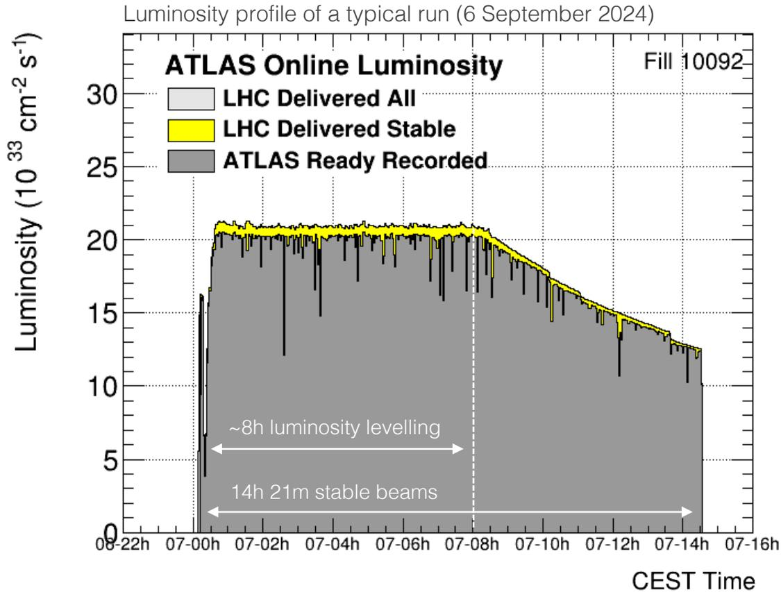
Luminosity levelling at  $2.1 \times 10^{34} \text{ cm}^{-2} \text{ s}^{-1}$  through defocusing and beam separation to keep pileup at ~63 until beam intensity has sufficiently dropped
