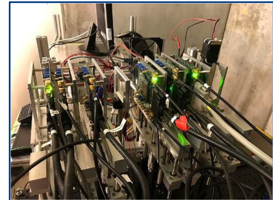
Characterization of potential electrode material with e^+ and \mu^+
