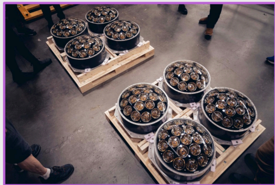
Multi-PMT photosensor modules and main electronics board
