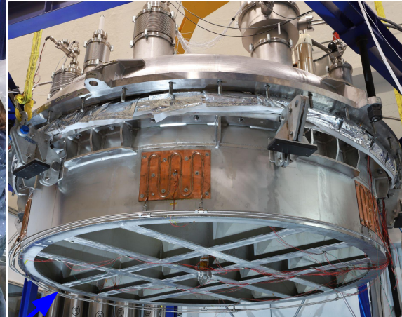
stiffening structure for flat floor
