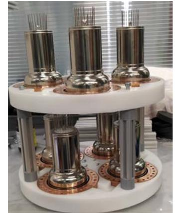
SiPM tracking plane with Teflon masks
