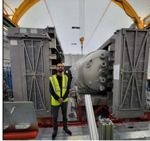
PMT energy plane installation with sapphire pressure windows
