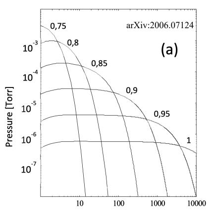
Outgassing in a vacuum chamber follows a power-law time dependence if there are multiple surface adsorption energy levels in the system
