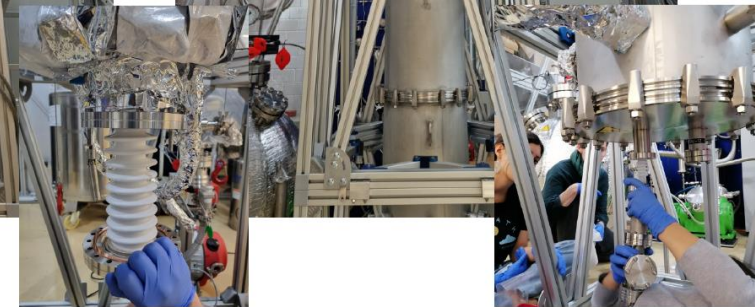
Close the outer cryostat and install high-voltage
