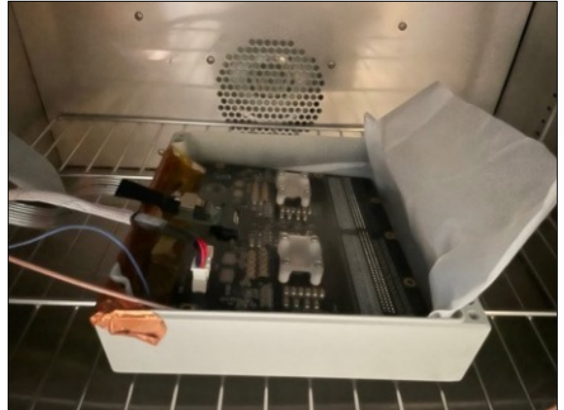
Environmental chamber cooled with LN2
