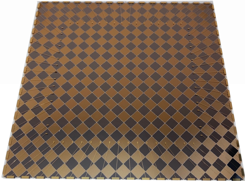
Vapor deposited electrode pattern on radiopure fused silica
