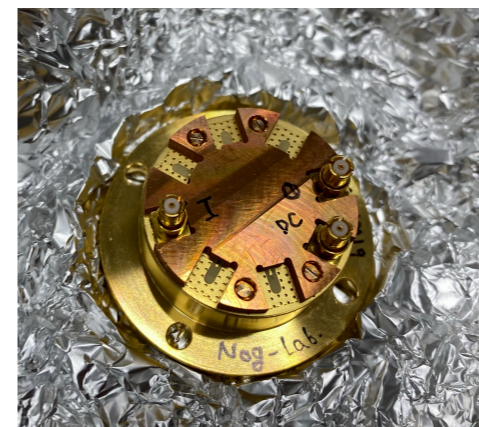
Metallic shield to suppress the spontaneous emission (2D impl.)
