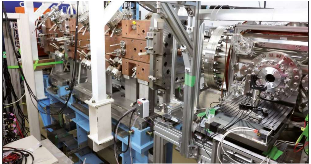
World first The experimental set up for muon cooling and acceleration at J-PARC. A beam of antimatter muons enters the apparatus from the right. Credit: J-PARC
