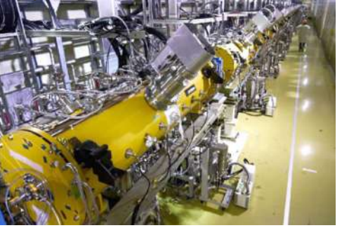
SDTL (Separated DTL) Up to 190 MeV
