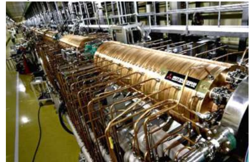
ACS (Annular-ring Coupled Structure Linac) Up to 400 MeV
