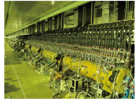
Drift Tube Linac (DTL) Up to 3 MeV
