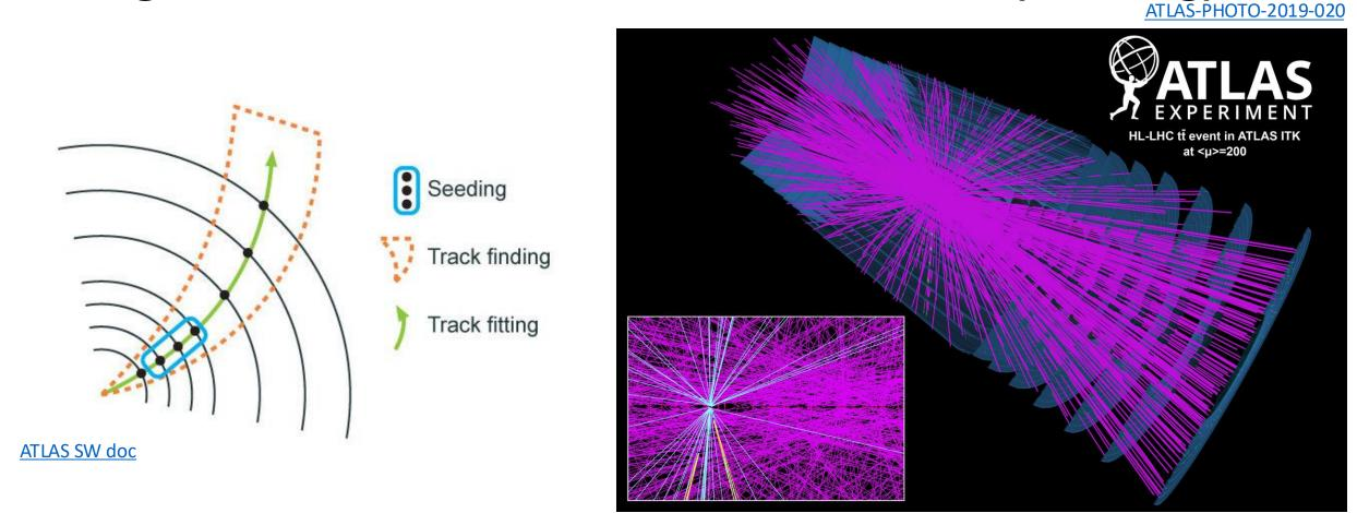
• Track reconstruction is a process of reconstructing the trajectories left by the charged particles by connecting the activated sensor space points.
